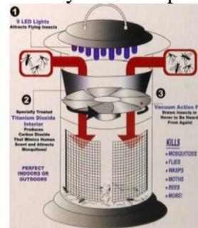
Figure 3: Design of solar trap fan for suck the pests
