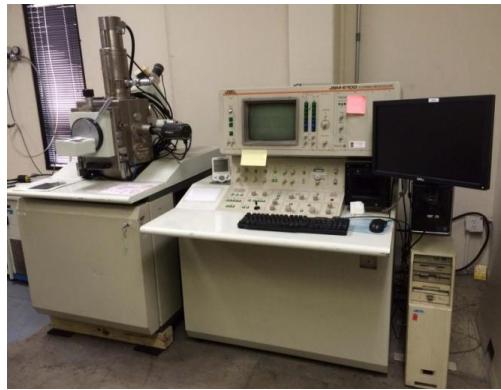
Figure- JEOL SEM Model JSM6100
