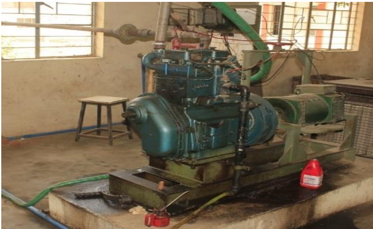
Fig. 1. Experimental setup with Catalytic converter attached to Exhaust line
